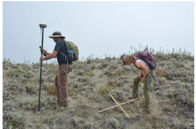
▲ Figure 35: Vegetation and RTK-GPS elevation surveys. Photo credit: Andrea Pickart.
