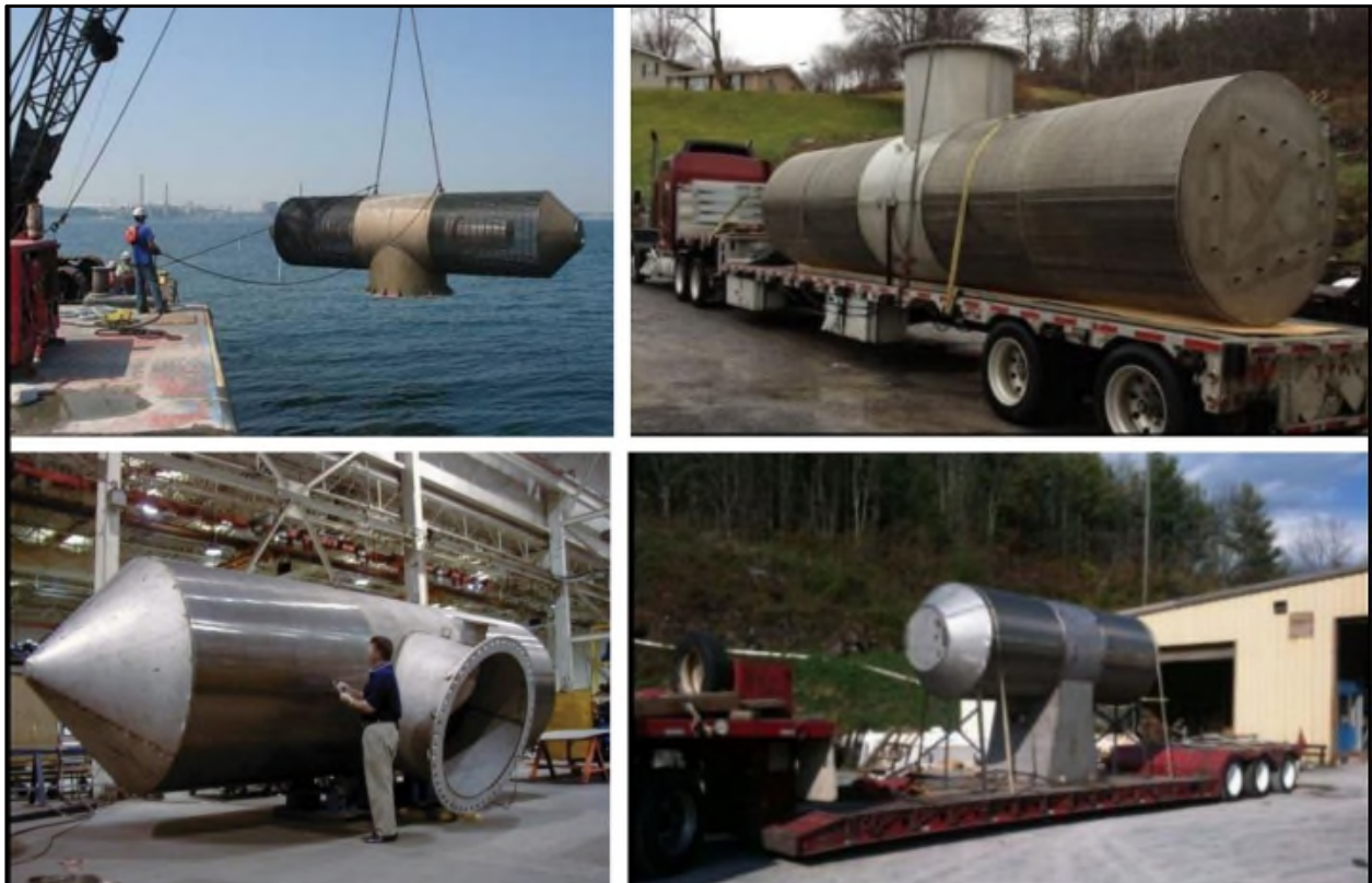
Figure 2-6. Wedgewire Screen Photographs
