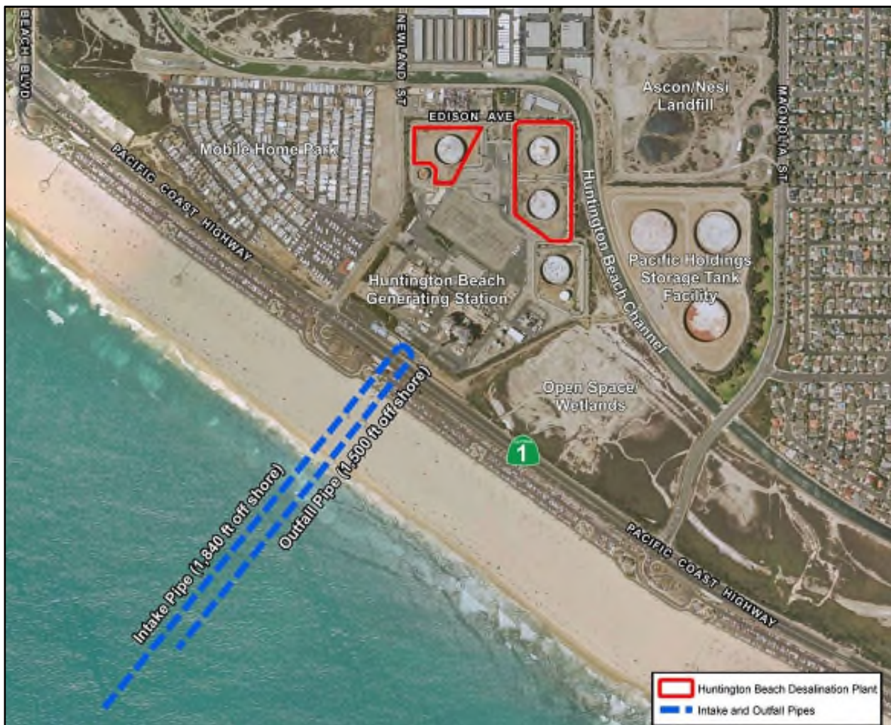
Figure 2-1. HB Desalination Plant with Intake/Discharge Pipelines
