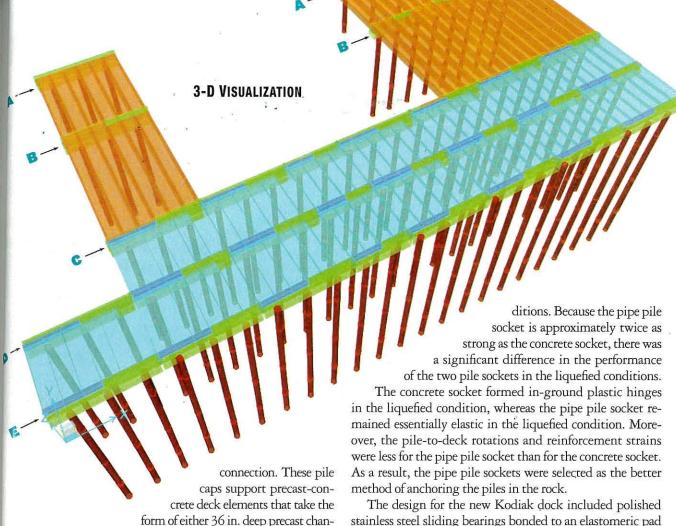
form of either 36 in. deep precast channel beams or 24 in. haunched precast deck panels. Cast-in-place concrete is used to integrate the deck elements and create a continuous pile cap. The abutment includes sliding bearing pads for the precast-concrete channel beams.
