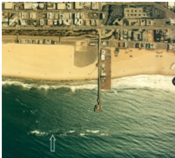
Offshore breakwater at the Santa Monica Pier. Note buildup of sand behind breakwater.
