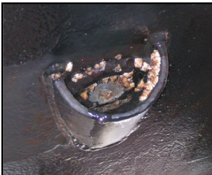
Figure V.1: Intake opening on a vessel hull.
