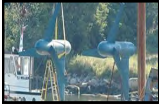
Figure 4.2.3. Kinetic Hydropower System by Verdant Power
