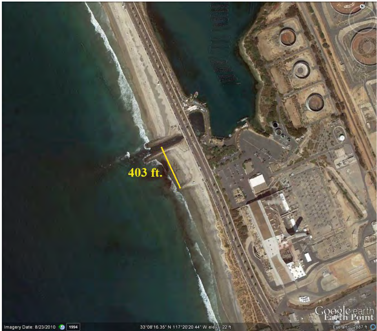
Figure 2: Google Earth image of the South Beach Groin presently located 403 ft south of the cooling water discharge channel at Encina Power Station, Carlsbad, CA.
