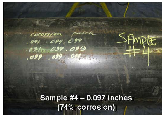
Figure 6– Photographs showing machined corrosion depths
