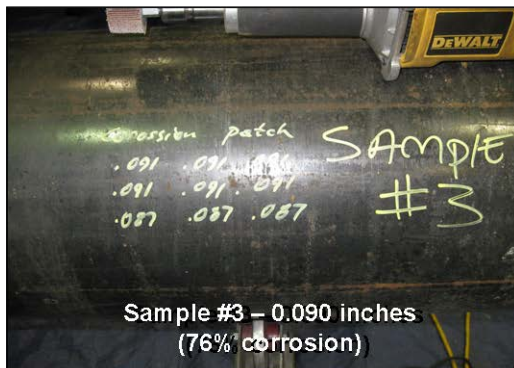
Figure 6– Photographs showing machined corrosion depths
