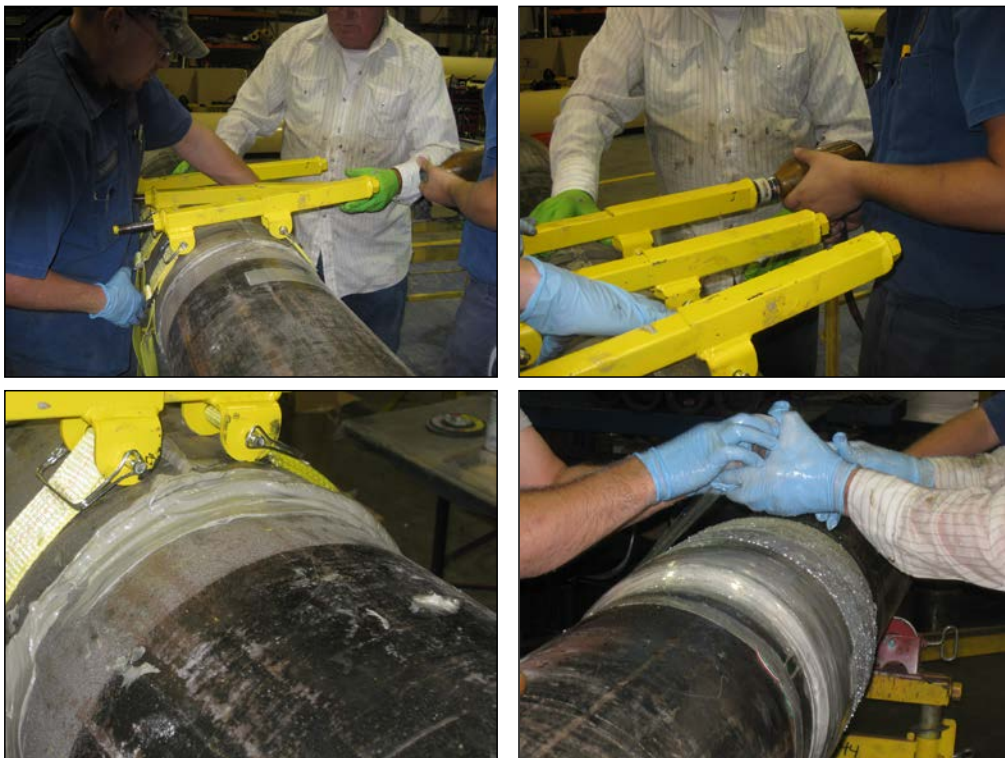
Figure 10 – Photographs of test sample preparation efforts (Set #4)
