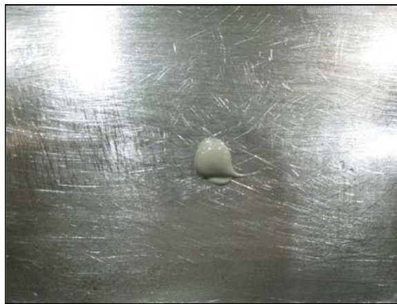
Figure 17 – Photographs of test sample having a thru-wall defect
