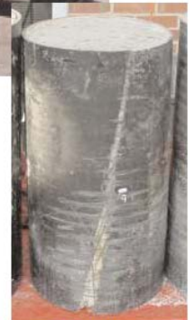
Axial failure mode
