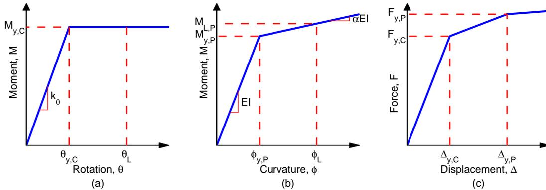
Figure 3. Idealized relationships: (a) Moment-rotation relationship of partial-moment-connection; (b) Moment-curvature relationship of the pile section; and (c) Force-deformation relationship of the pile system.
