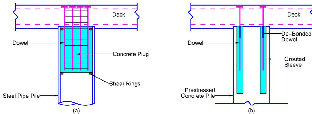
Figure 1. Partial-moment-connection of piles to the deck in marine oil terminals: (a) Concrete-plug connection for hollow-steel piles; and (b) Dowel-sleeve connection for pre-stressed-concrete pile.
