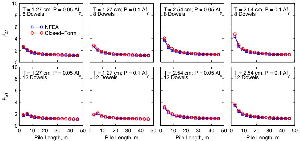
Figure 4. Displacement ductility capacity of hollow-steel pile at design Level 1.
