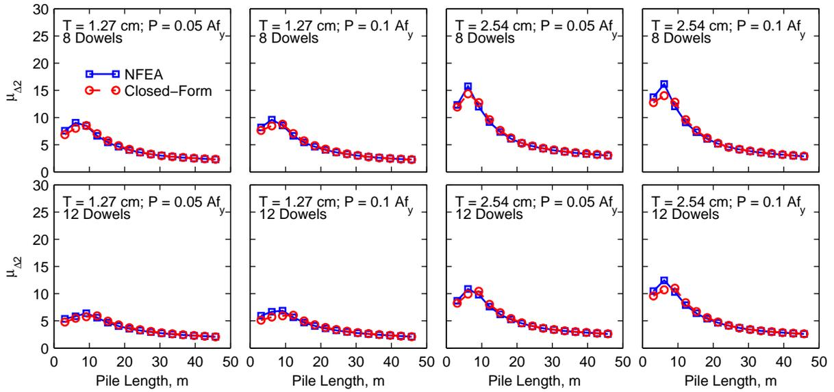
Figure 5. Displacement ductility capacity of hollow-steel pile at design Level 2.
