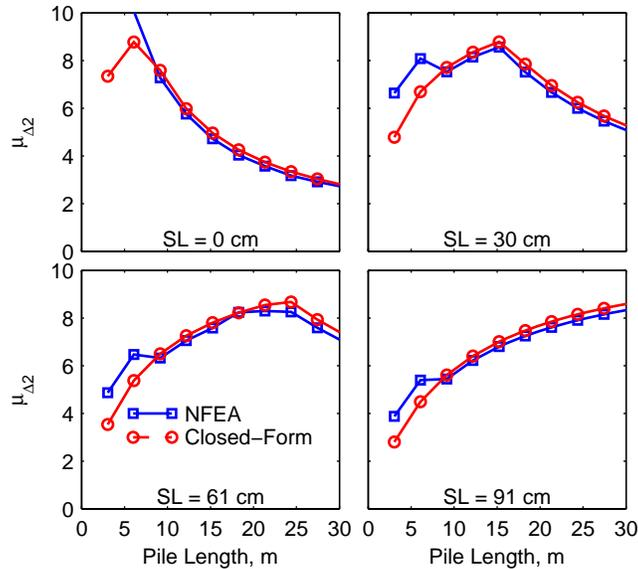
Figure 7. Displacement ductility capacity of pre-stressed-concrete pile at design Level 2.
