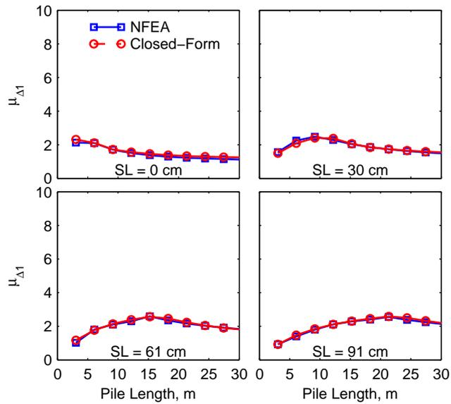
Figure 6. Displacement ductility capacity of pre-stressed-concrete pile at design Level 1.
