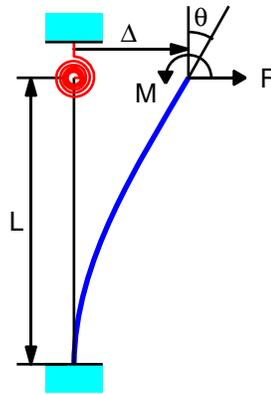
Figure 2. Simplified model of the pile with partial-moment-connection to the deck.
