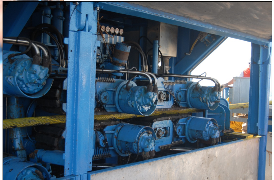
LCE hauling existing cable aboard.
