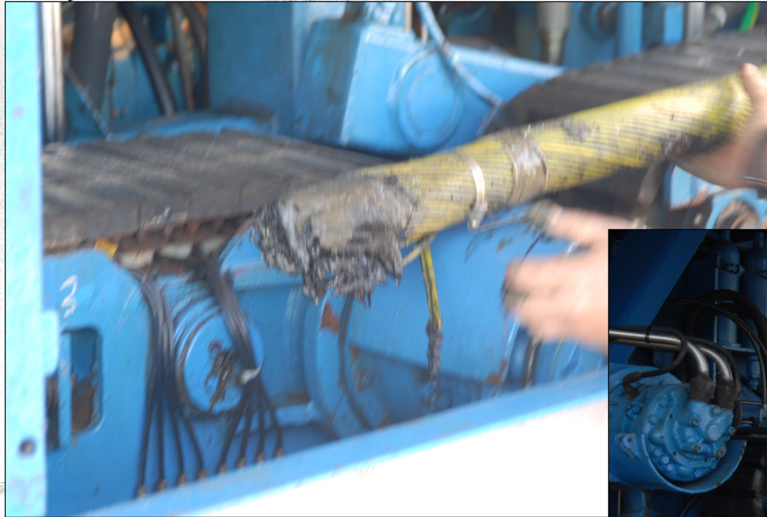
First cable cut in the LCE.
