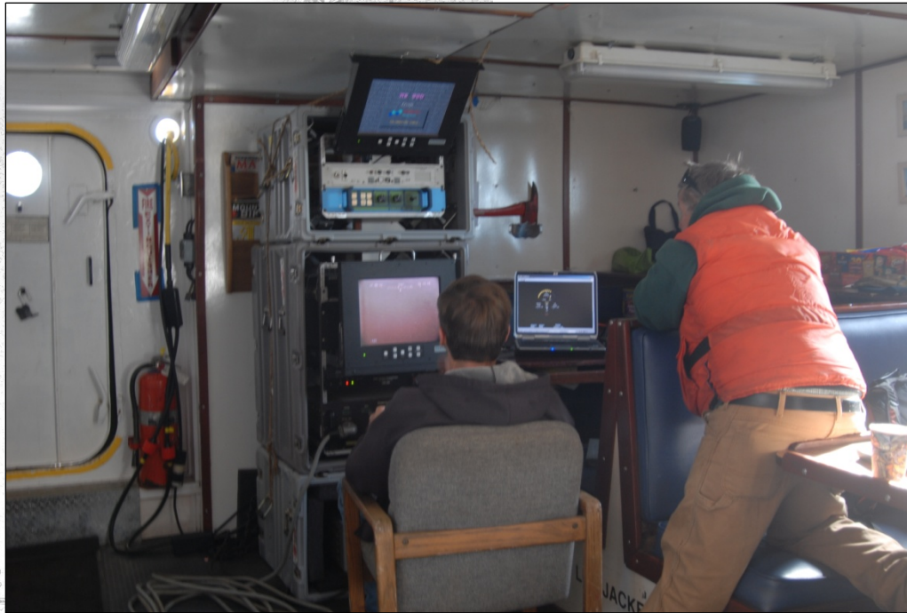
L3-Maripro ROV operator locating cable with cable tracker.
