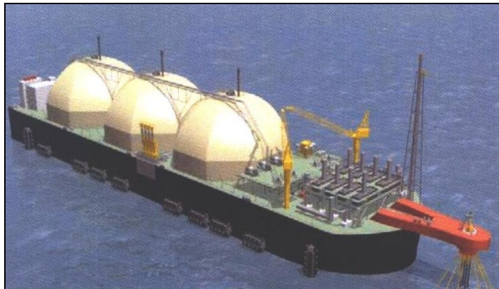
Figure 1. Conceptual design of the proposed Cabrillo Port LNG DWP Floating Storage and Regasification Unit (FSRU).
