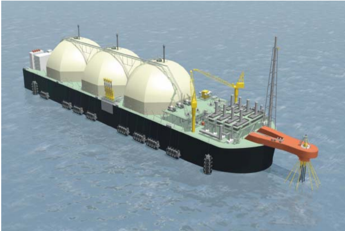
Figure 3: Floating Storage and Regasification Unit (FSRU) for Cabrillo Port
