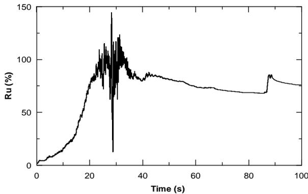
Figure 11 Excess Pore Pressure Ratio vs. Time nearby 9-Pile Group
