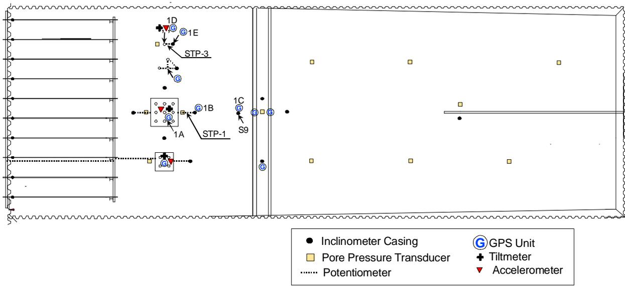
Figure 7 Instrumentation Plan for 1<sup>st</sup> Lateral Spreading Test
