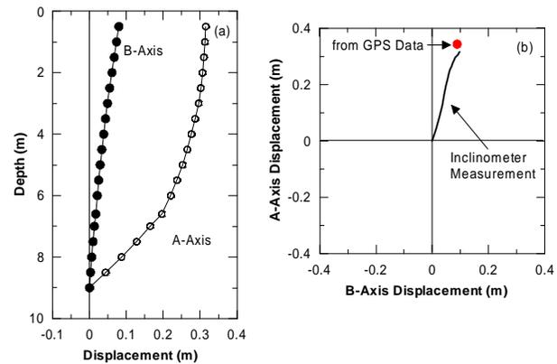
Figure 15 Soil Displacement Obtained from Slope Inclinometer Data (a) Section View, and (b) Plan View
