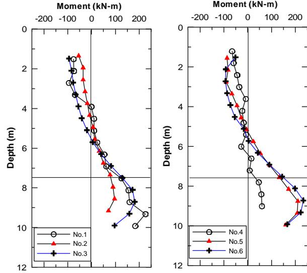
Figure 10 Moment Distribution of Each Pile in 9-Pile Group (Data Extracted from 1<sup>st</sup> Experiment)
