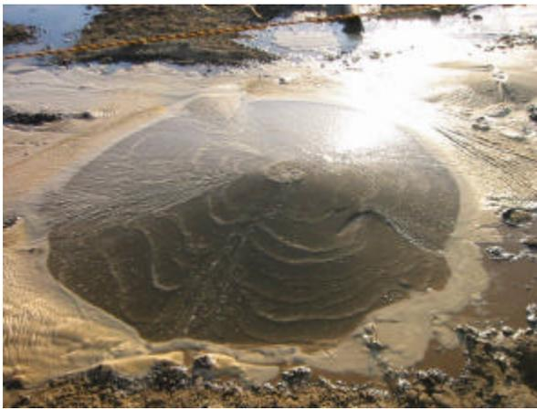
Figure 12 Sand Boil after the 1<sup>st</sup> Experiment
