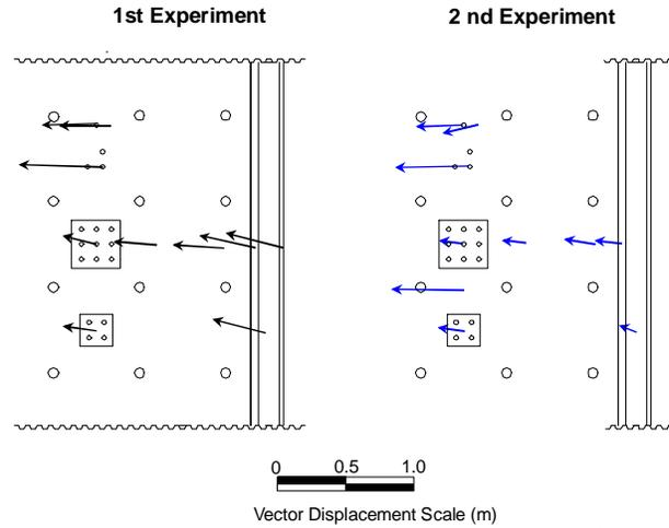
Figure 14 Vector Displacements from GPS Data for (a) 1<sup>st</sup> Experiment and (b) 2<sup>nd</sup> Experiment
