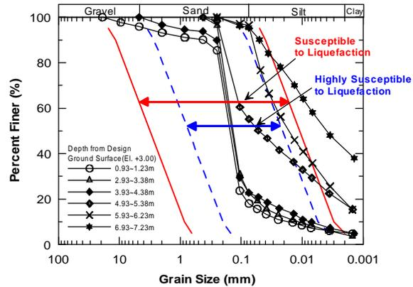
Figure 2 Grain Size Distribution of Soil at Test Site
