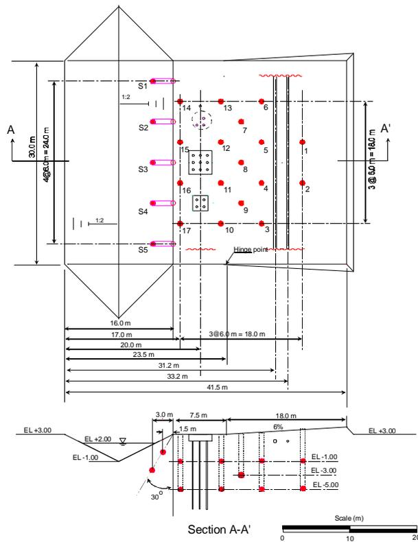
Figure 4 Site Layout of 2<sup>nd</sup> Lateral Spreading Experiment
