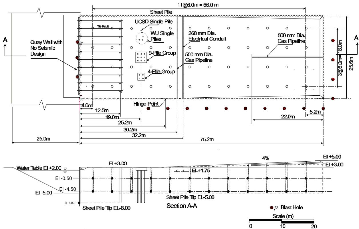
Figure 3 Site Layout of 1<sup>st</sup> Lateral Spreading Experiment
