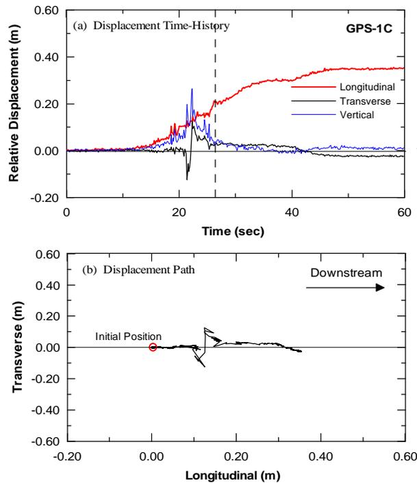
Figure 13 GPS Data (a) Displacement Time-History, and (b) Displacement Path
