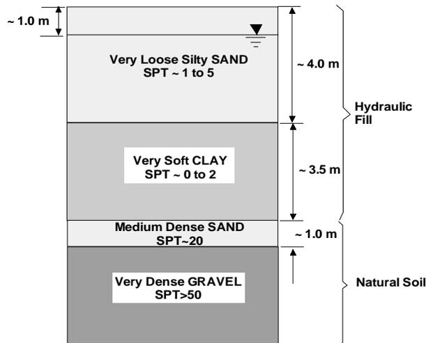
Figure 1 Typical Soil Profile of Test Site
