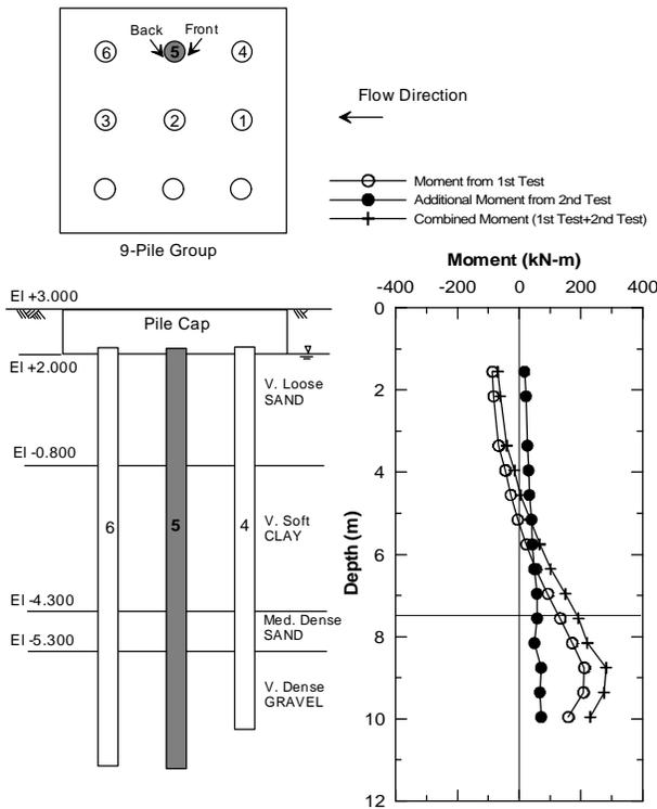
Figure 9 Moment along Pile No.5 of 9-Pile Group
