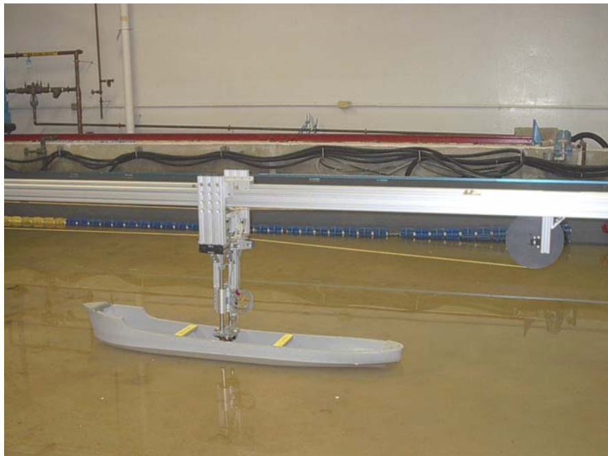
Figure 3b. View of towing carriage attached to drive cable.
