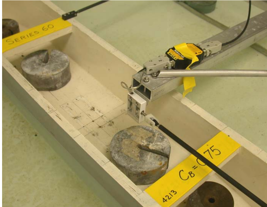
Figure 7. View of load cell used to measure mooring loads.
