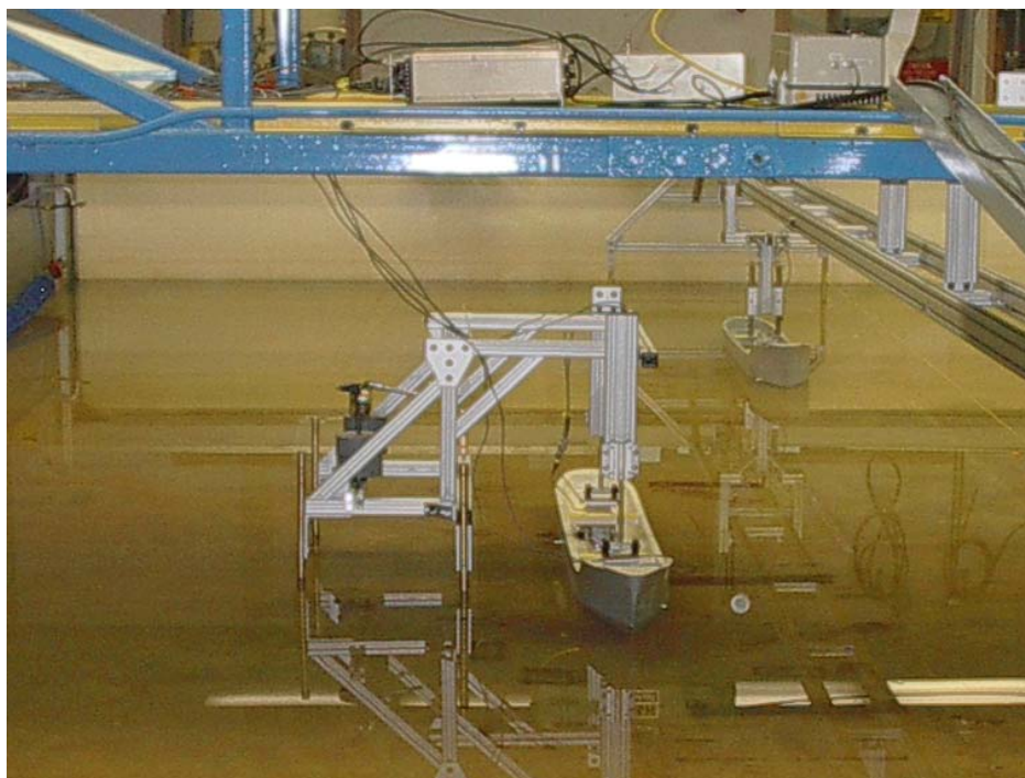
Figure 5. Original test frame used to measure mooring loads, viewed from front
