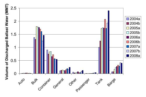
Figure V.11. Volume of Ballast Water (million metric tons; MMT) Discharged per Six-Month Period as a Function of Vessel Type. (a = January to June, b = July to December)
