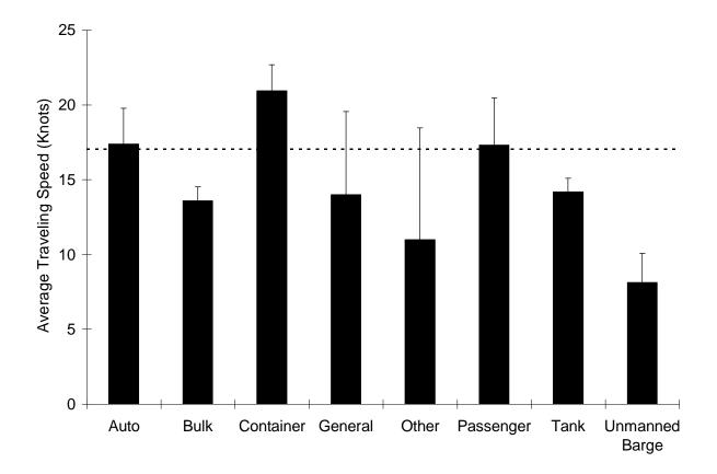
**Figure V.30.** Average (<u>+</u> standard deviation) Traveling Speed (knots) for each of the Vessel Types Operating in California. Dotted line represents the average speed of the California fleet as a whole.
