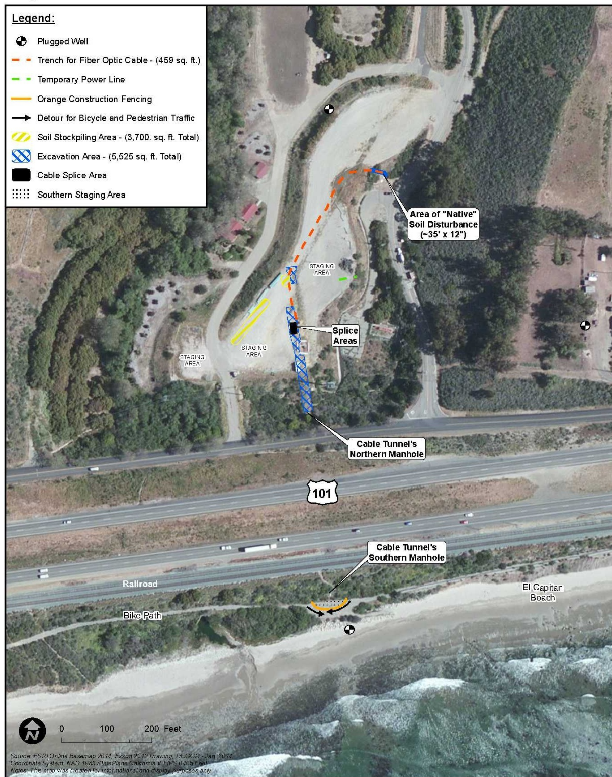
Figure 3.12-1. Plugged Wells Within/Adjacent to Onshore Construction Area
