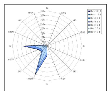
Figure 4.3-3. Wave Rose for Oceanside Buoy CA045 (May 1997 to July 2003). Adapted from BGI 2003.
