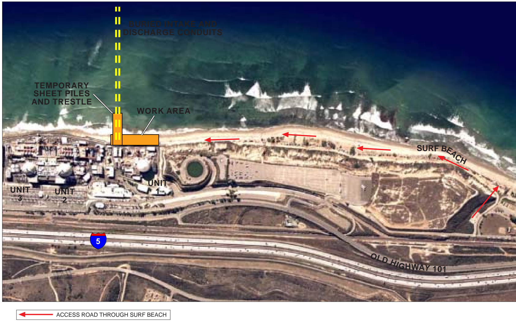
Figure 3.3-1 Aerial View of Onshore Components Complete Removal of Conduits Alternative
